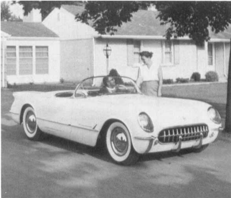
FIG. 20. The 1953 Chevrolet Corvette was the first production car with a fiber glass body, molded by Molded Fiberglass Co.
