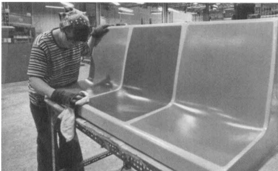
FIG. 22. Transit bus and subway seats made of FRP.
